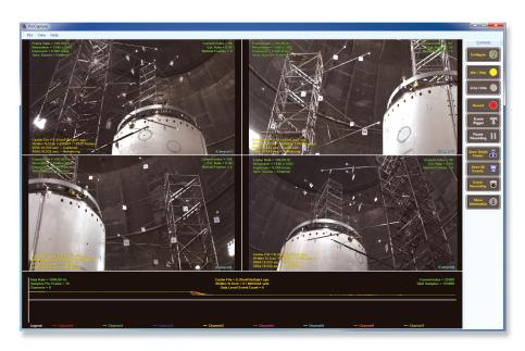
The ProCapture control panel allows users to configure settings and switch between Live, Record, Event Trigger, or Save at the touch of a button. Overlay information displays the settings instantly.
